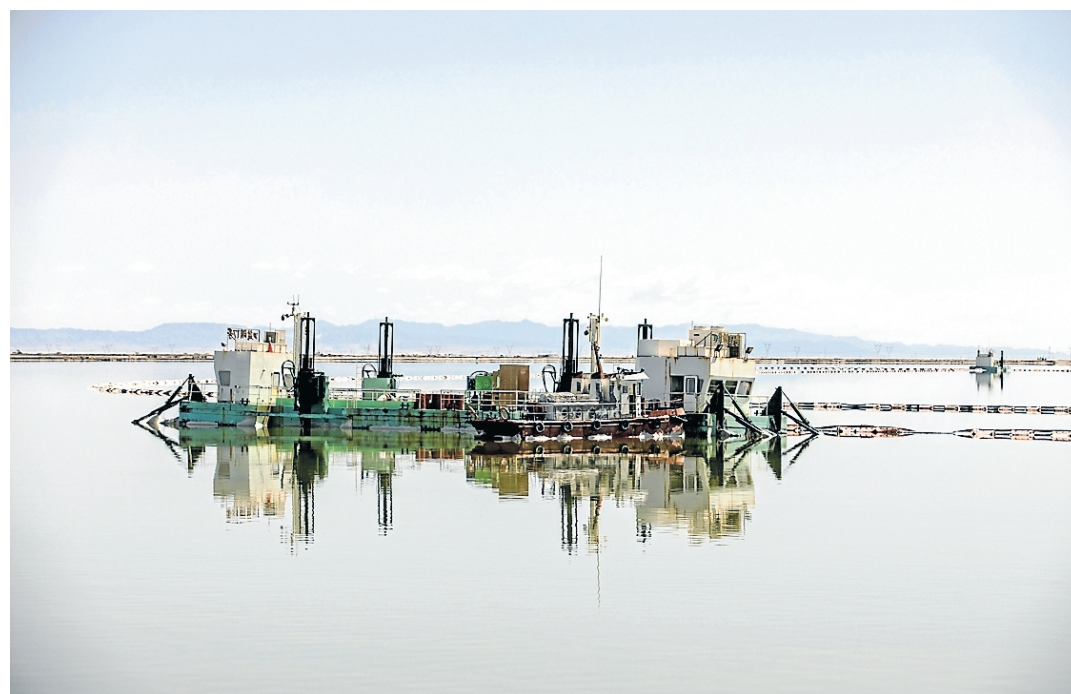
A pumping barge floats on a salt lake retention pond at the Qinghai Salt Lake Group in Golmud. PHOTO: QILAI SHEN
