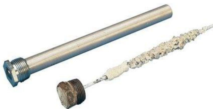
Figure 8 – Sacrificial anode: New vs. Corroded
